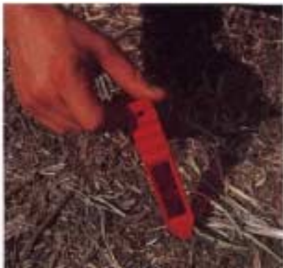
An in situ measure of PRS™ soil nutrient supply rates allows researchers to measure another “piece of the nutrient supply puzzle”.
