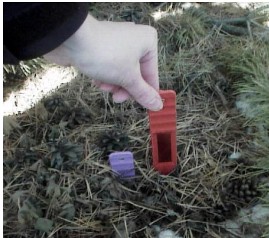
Figure 1. PRS™-probes: an effective tool for measuring forest soil nutrient dynamics in situ .
