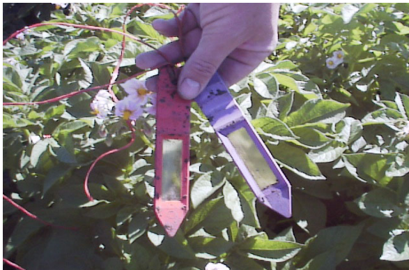
Figure 1. PRS™-probes (orange and purple probes are anion- and cation-exchange probes, respectively) used to measure the effects of different organic amendments on soil N supply in dryland potato production.
