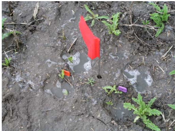
Figure 3. PRS™-probes used to measure the effect of broadcasted liquid hog manure on soil nutrient availability. (Photo courtesy of Dr. Ken Van Rees)
