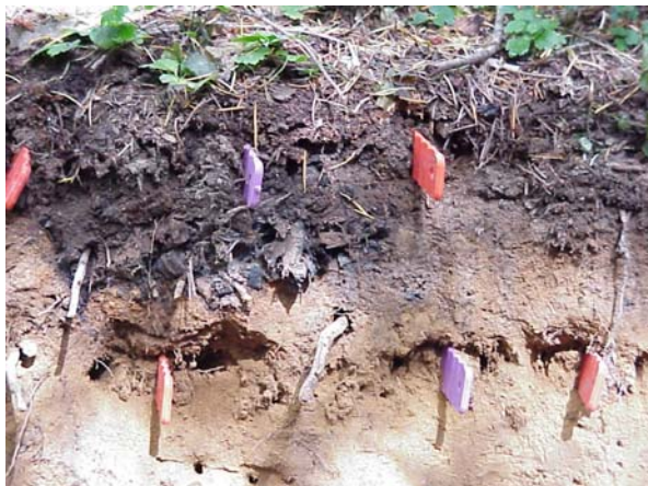
Figure 1. Anion- (orange) and cation-exchange (purple) PRS™-probes used to measure temporal changes in nutrient availability throughout the growing season in different soil horizons. (Photo courtesy of Dr. Mariann Garrison-Johnson)
