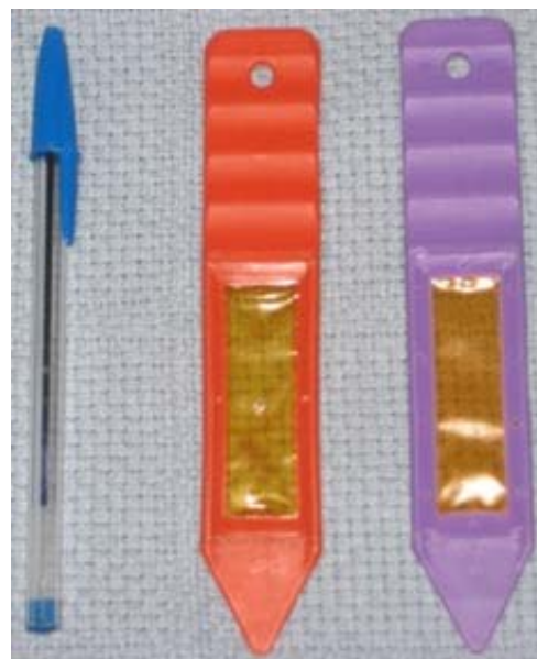
Figure 3.1 A PRS TM -probe pair consists of one cation (orange) and one anion (purple) PRS TM -probe.
